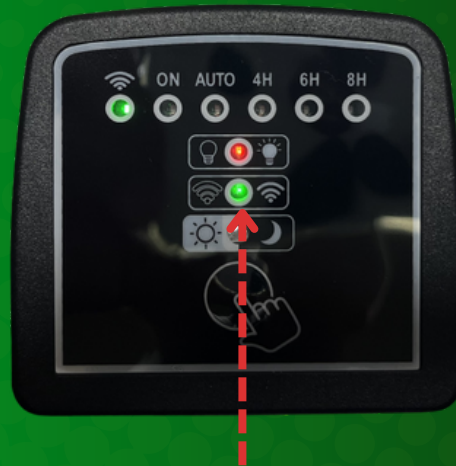
During setup, the transformer's LED blinks to indicate it is connecting to Wi-Fi
