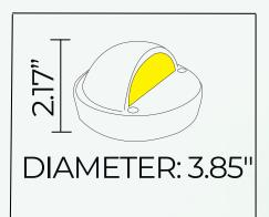
**POWER: FINISH:** BLACK INTEGRATED 3W LED 12V AC/DC 3000K OR 5000K **FEATURE: BODY:** SURAFCE MOUNT HEAVY DUTY CAST ALUMINUM **CERTIFICATE: INCLUDED: ETL LISTED** 20" INCHES WIRE **STA09LED SPEC SHEET** www.ABBALightingUSA.com
