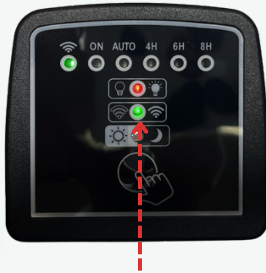
During setup, the transformer's LED blinks to indicate it is connecting to Wi-Fi
