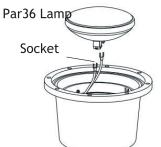
Insert the lamp with the correct wattage and type marked on the fixture label.
