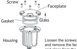
Loosen the screws and remove the faceplate, gasket, and glass from the housing.
