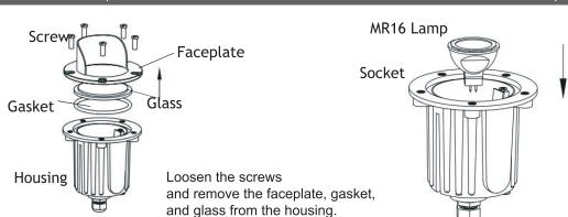
Insert the lamp with the correct wattage and type marked on the fixture label.
