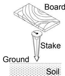
Determine the desired location for mounting the luminaire. Hammer the stake into the ground until flange of stake is flush to grade. To avoid damage to the stake, place a board on top of the stake while hammering.
