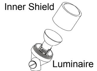
Thread the inner shield onto the luminaire and hand tighten until snug.
