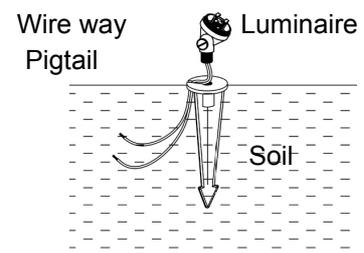
Clear away an area in the ground at the wire way on top of the stake. Lay the luminaire pigtail into the wire way and attach the luminaire onto the stake. Tighten until snug.
