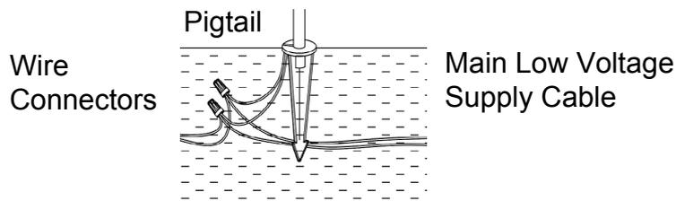
Strip both leads from the luminaire pigtail. Using two wire connectors (sold separately) connect the leads from the luminaire to the main supply cable leads.
