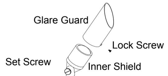
Place the glare guard onto the inner shield and secure it with the lock screw. Adjust the luminaire to the desired angle by using the set screw.
