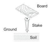
Determine the desired location for mounting the luminaire. Hammer the stake into the ground until flange of stake is flush to grade. To avoid damage to the stake, place a board on top of the stake while hammering.
