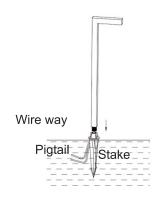
Clear away an area in the ground at the wireway slot on top of the stake. Lay the luminaire pigtail into the wireway slot and screw the stem onto the stake. If the fixture does not look straight, adjust by pushing or pulling on the stake only.
